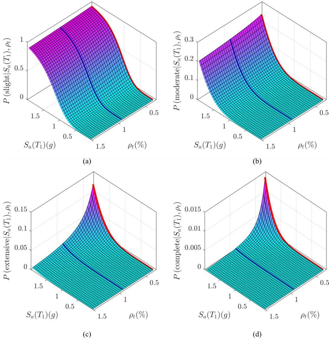
Figure 4. Fragility surfaces for columns conditioned on spectral acceleration and transverse reinforcement ratio for (a) slight, (b) moderate, (c) extensive, and (d) complete damage states. Red and blue lines indicate transverse reinforcement ratios for as-built and according to current Canadian design requirements, respectively.
