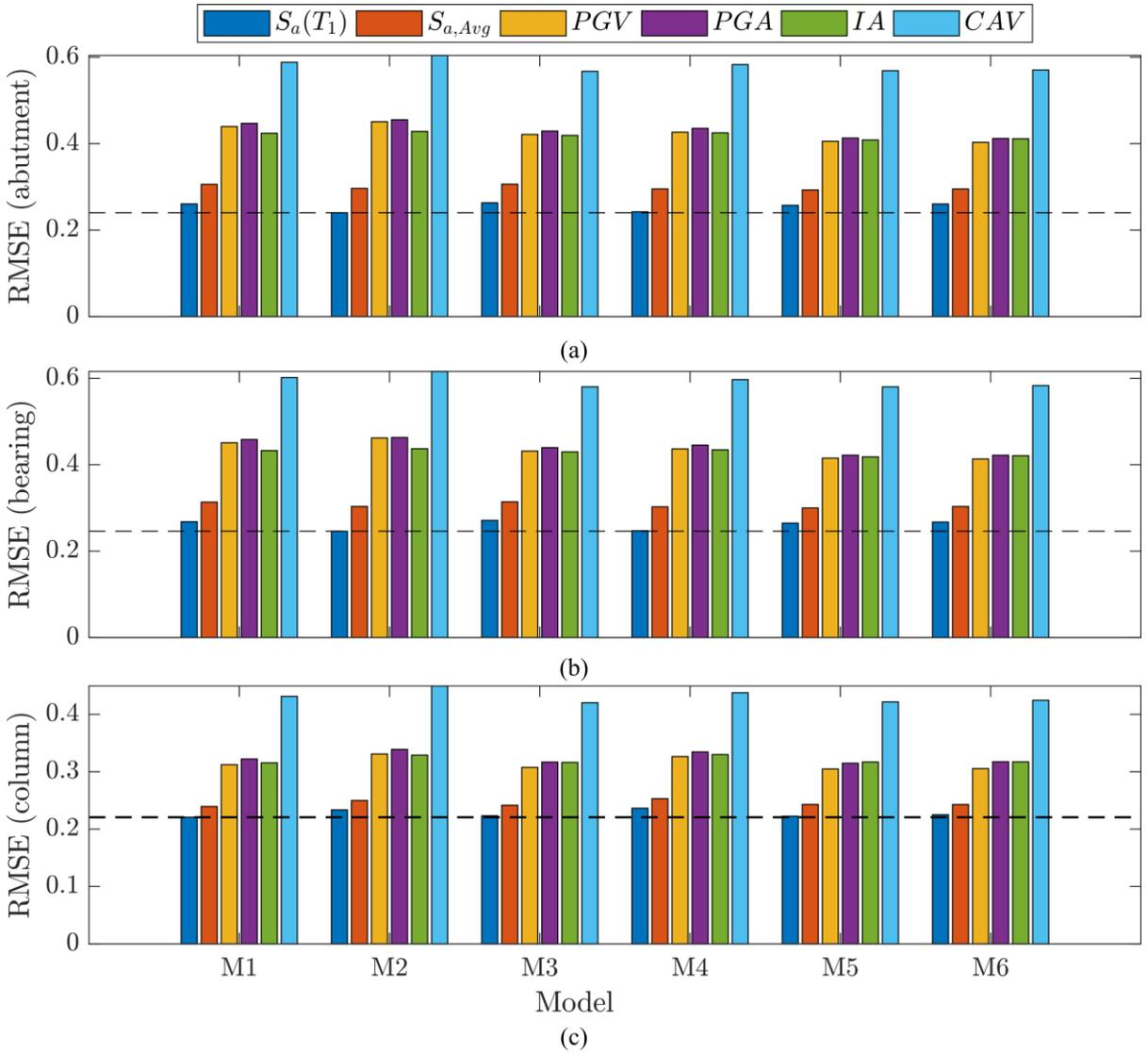
Figure 2. Comparison of performance of metamodelling with different intensity measures from 10-fold cross-validation for: (a) deformation on abutment wing walls, (b) deformation on elastomeric bearings, and (c) column drift. Dashed lines indicate lowest root mean squared errors.
