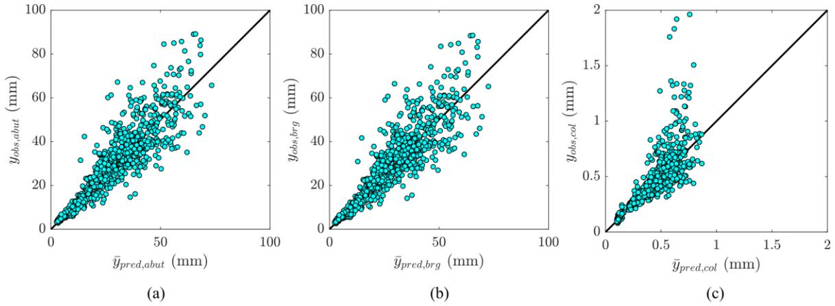
Figure 3. Comparison of observed and predicted responses for (a) abutments, (b) bearings, and (c) columns.
